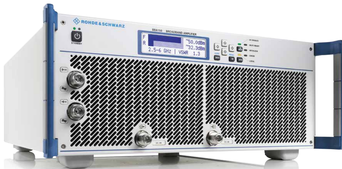
Fig. 1: The new R&S® BBA 150 broadband amplifier models provide power levels from 15 W to 200 W at frequencies between 2.5 GHz and 6 GHz.
