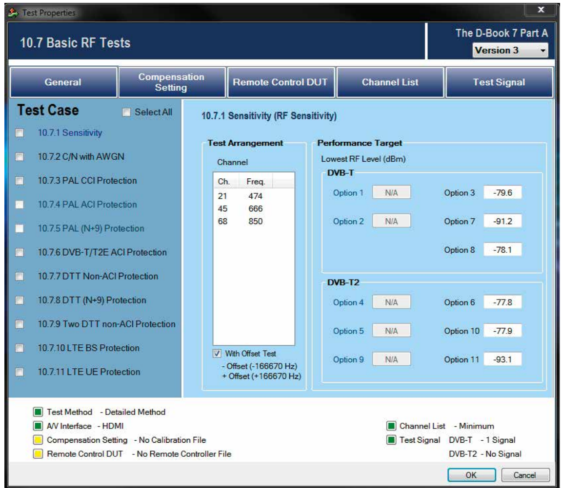
Fig. 8: Automation reduces test times and delivers reproducible results. This example shows the D-Book Minimum Requirement Specifications test case.
